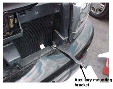
4 - Place the grillguard up to the bottom mounting brackets and secure into place using ½ x 1 ½" hex head bolts, flat washers, and lock nuts.
