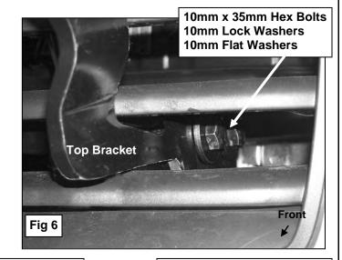
Pull the Top Bracket as the hardware is tightened to provide maximum clearance between Grille Guard and vehicle
