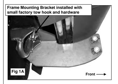
The heavy duty factory tow hooks cannot be reinstalled and will not clear the Frame Mounting Brackets
