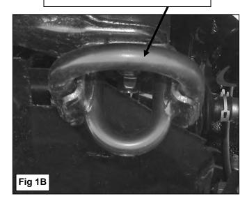
Insert Double Bolt Plate through the back of radiator core support cross member
