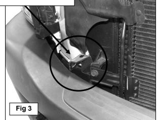
(1) 10mm x 35mm Hex Bolt (2) 10mm Flat Washers (1) 10mm Nylon Lock Nut
