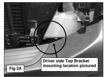
Use the 8mm factory hex bolt to attach the Top Mounting Bracket to the crossmember
