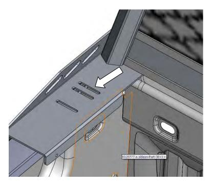
Should your Cab Rack not have any of the available slots line up with the stake pocket holes, or the available slots do not allow the rubber mounting block to insert properly, omit the rubber mounting block from Step 3 and try again. You may also need to drill a hole into the Cab Rack to properly line up with the stake pocket hole.
