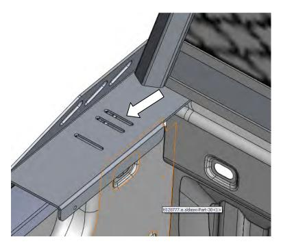
Should your Cab Rack not have any of the available slots line up with the stake pocket holes, or the available slots do not allow the rubber mounting block to insert properly, omit the rubber mounting block from Step 3 and try again. You may also need to drill a hole into the Cab Rack to properly line up with the stake pocket hole.
