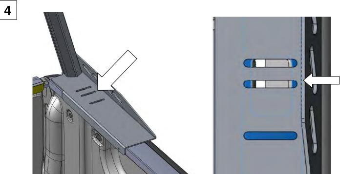
Note: If your Cab Rack does not line up with a stake pocket hole, refer to end of installation Instruction
