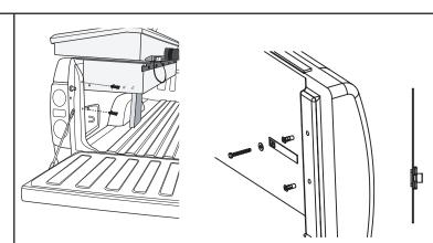
Drill 1/2" holes at the marks in the corner post. Install riv-nuts in the 1/2" holes using the supplied wrench.
