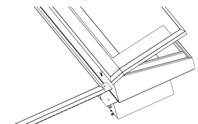
Bolt the Tonneau cover to the Tonneau rails with carriage bolt thru the holes in the front of the rail.
