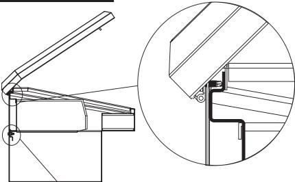
1: Insert bracket into top channel at desired location on top of toolbox between screw and inside bend, if using 5.5" bins install bracket with the 4 slots on top if using 4" bins install the bracket with the 5 slots on the top.
