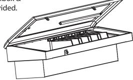
3: Install foam bumper strip on the interior pan 6" back from the front edge and over the top of the bins. Wipe pan clean before installing.
