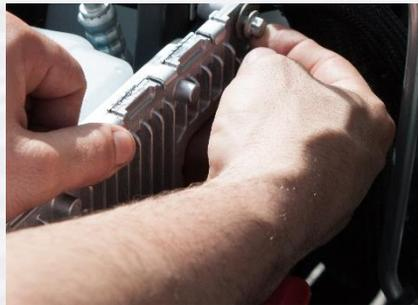
6. Remove upper PCM connector first by pressing center button and sliding lock back words away from the computer wiggle if tight do not force red clip. Follow this by the bottom connector.
