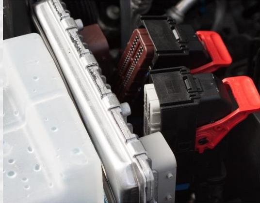
7. Remove the stock PCM from the engine compartment.
