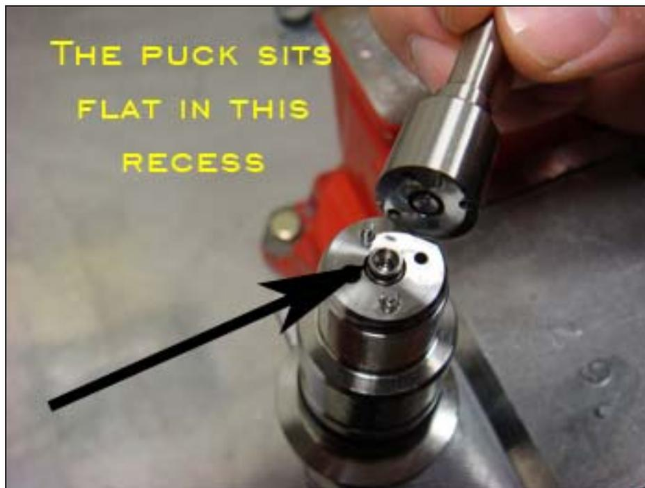
**7. Clean nozzle and injector body mating surface to remove any carbon that may have fallen on the mating surface during disassembly. You may use brake clean but DO NOT blow the puck out of the hole, or remove it before spraying.**
