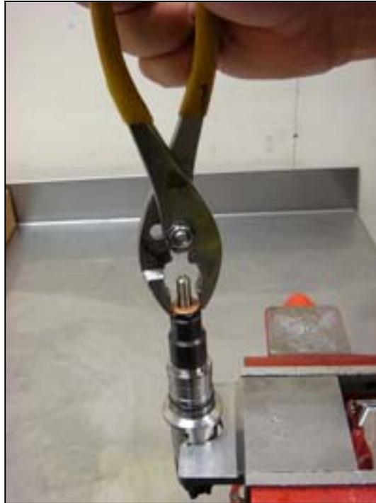
**6. Using a 15mm wrench, remove the nozzle cap. Once you have removed the nozzle cone you can remove the nozzle, but **BE CAREFUL** not to lose the small puck which can sometimes stick to the nozzle. The puck fits into the small recess right in the middle of the injector body and lays flat.**
