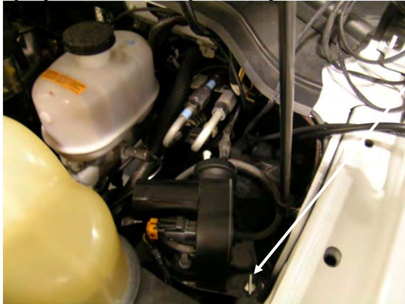
Twist tab to remove the vacuum pump. Lift the pump up and outwards to remove.
