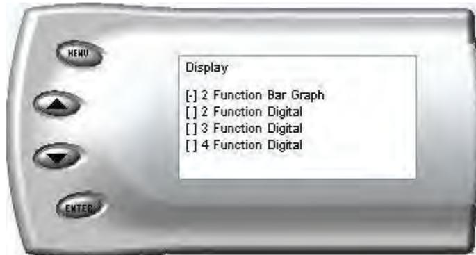
3. Select the desired viewing option by using the up and down arrows and pressing the [Enter] key. Below are examples of the display options:
