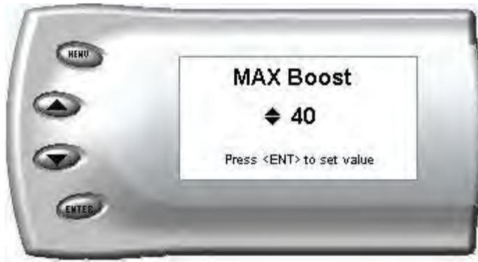
2. Change the Max Boost set point by pressing the up and down arrow keys to select the maximum pounds of boost that the turbo is allowed to produce. Once the number is set, press [Enter]. When the boost level reaches this value, the power delivery will be reduced so as not to allow the boost to exceed this set value.
