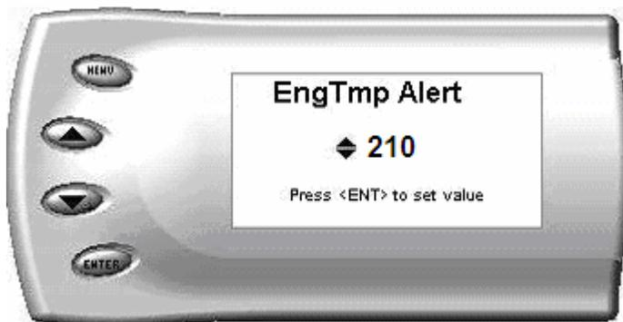
8. Press the up and down arrow keys until you see the desired Engine Temp level at which you want to be alerted and press [Enter] to set that value.
