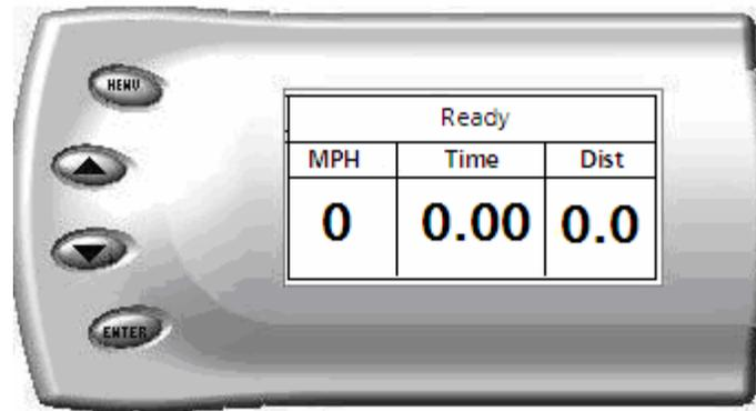
The monitor screen will then flash 3 times to simulate the lights at a drag strip, then when you get the green light the monitor will display “GO” at the top of the screen.
