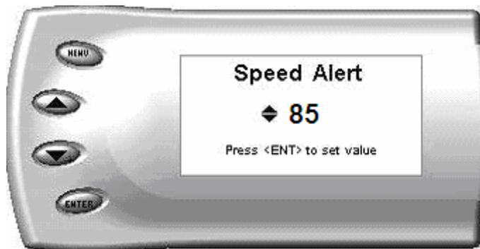
12. Press the up and down arrow keys until you see the desired Speed at which you want to be alerted and press [Enter] to set that value.
