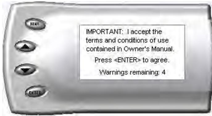
Press the <ENT> key to accept the terms and conditions in your Owner's Manual. A screen similar to the following appears indicating that your Juice and Attitude were installed correctly.
