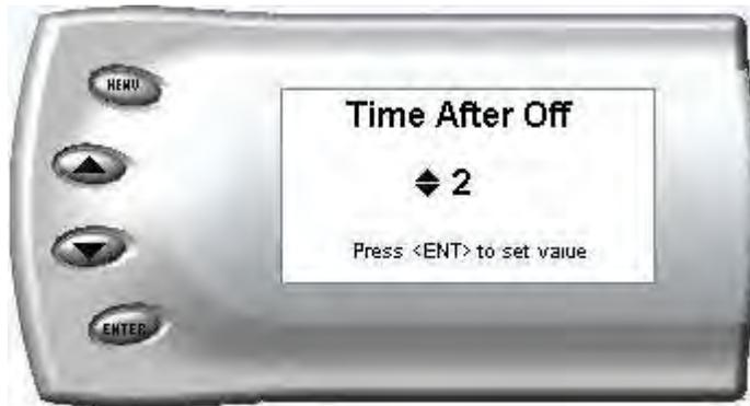
**NOTE: The turbo timer will not function when the truck is regenerating.**
