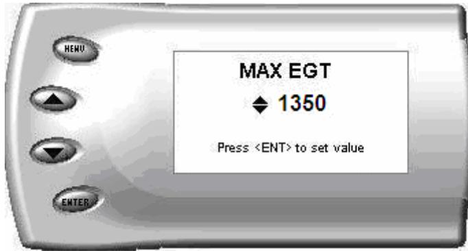
Change the Max EGT set point by pressing the up and down arrow keys to select the maximum temperature that you want the exhaust gas temperature to reach, then pressing [Enter]. When the exhaust gas temperature reaches this value, the power delivery will be decreased so as not to allow the temperature to exceed this set value.
