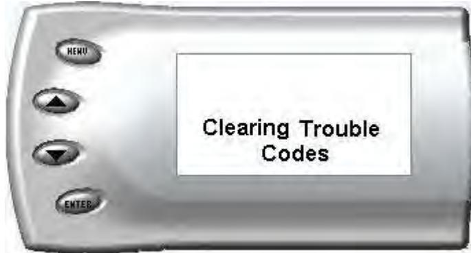
**Note:** After clearing trouble codes you may notice a P-1000, code displaying in your moitor, this error occurs when all other DTC's have been erased from the system. This error will subside when all OBD monitors have been completed.
