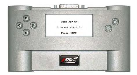
14. After pressing <ENT>, the *Evolution* tests the PCM for communications. If successful, a truck does a "Burnout" and the FINISHED screen appears:
