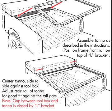
Place clamps 12" from each end. Center the middle clamp between the other two. Tighten clamps and install bows and tonno per the install sheet.
