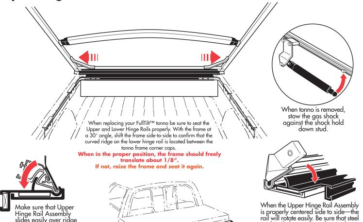
If you need to tow your vehicle backward, be sure to release the cover and stow against the hinge rail using Velcro® straps provided.
