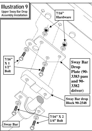
Torque according to the torque chart. Use thread locker on these bolts. See ILLUSTRATION 7.
