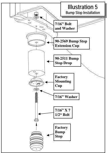
suspension kit instructions for coil spacer block assembly.
