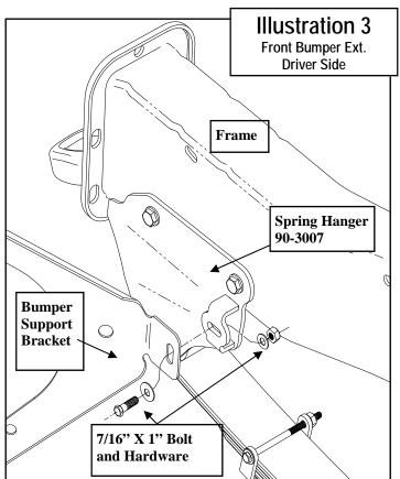
of spring to remove the factory front spring hanger. Save all hardware for reuse
