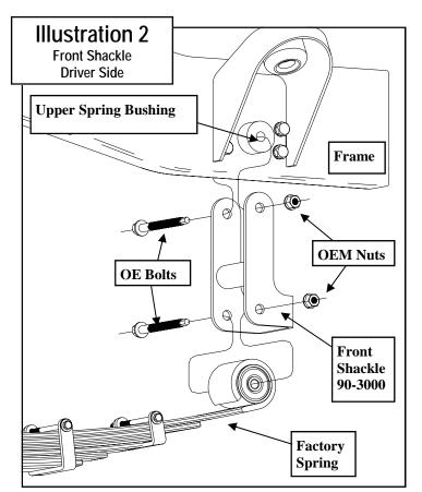
TECH TIP: Factory spring bolts are secured with loctite which makes removal difficult. By warming the nut with a propane torch to approx. 300 degrees Fahrenheit the loctite will release and the hardware can be removed with hand tools.
