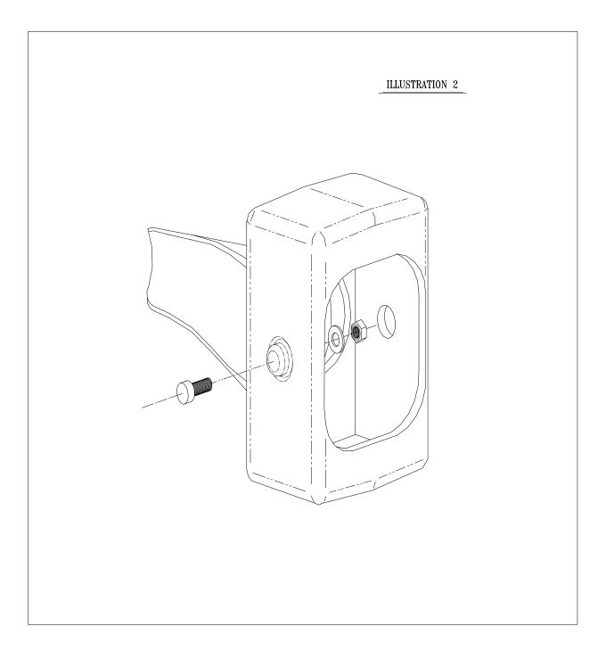
7) Install the block(s) and raise the axle to install spring center bolt into the hole in the top of the block.
