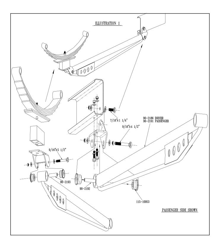
If vehicle is equipped with a ProComp Suspension and the billet aluminum block was installed, check the alignment pin to be sure there is 1/2" of pin protruding from the block. Place the aluminum block on top of the axle bracket and align the pin with the hole in the bracket and the hole in the spring pad.
