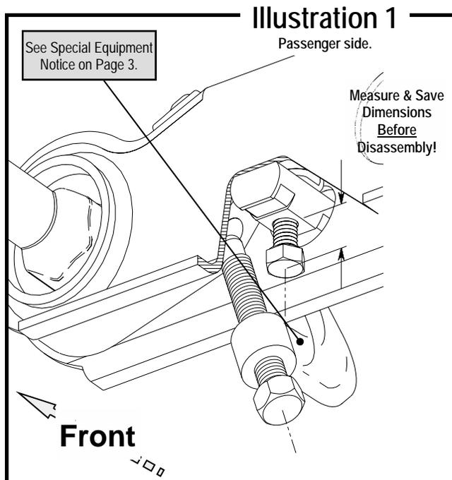
**Note:** If the bar seems stuck, use a hammer and punch through the hole in the rear of the cross member to dislodge it.
