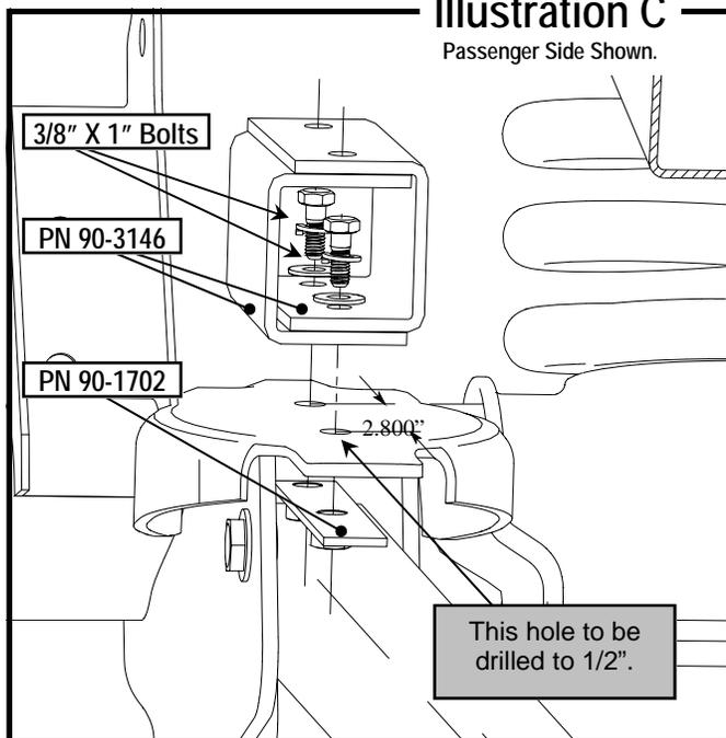
with lock washer into the remaining nut on the nut plate. Tighten these bolts to 45 ft-lbs
