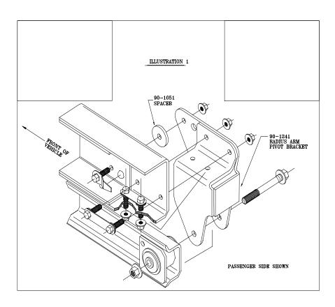
7) Remove passenger radius arm pivot bolt at the bracket. Remove the hardware securing the bracket to the frame and remove bracket.
