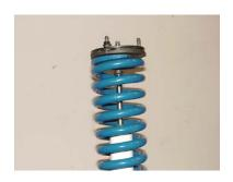
4. Take the stock strut assembly place into a vise, then use the external coil spring compressor to compress the spring enough to remove top nut. **WARNING: COIL SPRING IS UNDER EXTREME LOAD.** Remove the top nut and remove stock isolator mount, discard stock coil spring and shock.
