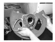
6. You will not be reinstalling the dust shield on the lift spindles, but on trucks with front ABS you will have to separate the ABS sensor from the dust shield so that it can be reinstalled onto the lift spindle.
