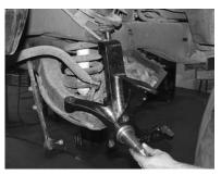
Take the driver's side spindle, marked FT2588-7D, and install it onto the upper and lower ball joints. Reinstall the original castle nuts and torque to factory specs. Install a supplied cotter pin in each castle nut, DO NOT REUSE THE ORIGINAL COTTER PINS.
