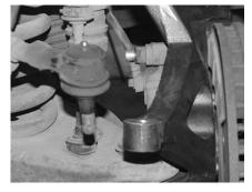
8. Loosen the tie rod adjuster clamps and rotate the tie end a ½ turn so it can be reinstalled from the top of the spindle. Retorque the original castle nut to factory specifications and install a new cotter pin.
