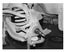
3. Remove the nut securing the tie rod end to the spindle. Use a ball joint puller to separate the tie rod end from the spindle. Remove the dust cap from the rotor, remove the cotter pin and nut from the axle and slide the rotor off the spindle. Keep the wheel bearings
