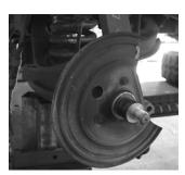
3. Remove the nut securing the tie rod end to the spindle. Use a ball joint puller to separate the tie rod end from
