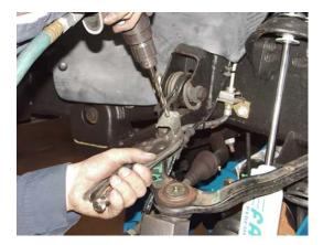
9. Locate the lower shock mount and place over the factory upper control arm. Using 3/8" x 2" cross bolts, nuts and washers attach arm with the brake hose retaining clamp to the inside of the control arm. Note must use 3/8" x 2" bolts on the mount eyes closest to frame to allow for shock clearance. Use 3/8" x 2-3/4" bolts, nuts and washers for the mount holes to the outside of the vehicle under the control arm. Leave all bolts loose. SEE BELOW PHOTOS
