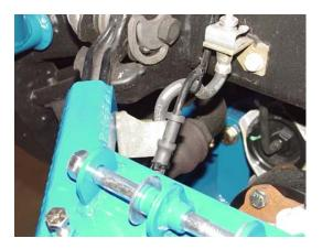
10. Locate and thread 3/8" x 1-1/2" bolt with thread locking compound into the welded nuts on the top of the lower shock mount and tighten against the stock control arm. Snug up bolts only, do not over tighen.
