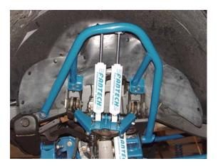
13. Repeat same procedure for passenger side. Except step 2, remove the factory differential mounting bolt on the side of the frame rather than the steering box bolt. For ease of installation cut 5/8" off the end of the rear differential mounting bolt that protrudes through the frame. Follow all other steps the same as the driverside.
