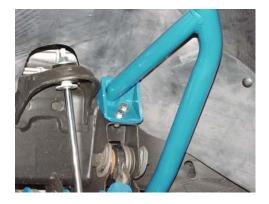
7. Tighten the steering box bolt to 90LBS and the lower control arm rear bolt to 90LBS
