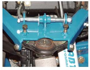
12. Locate and install Fabtech shocks part number FTS7052 using  $\frac{1}{2}$  x 5-3/4" bolts, nuts and washers. Torque bolt to 35LBS.
