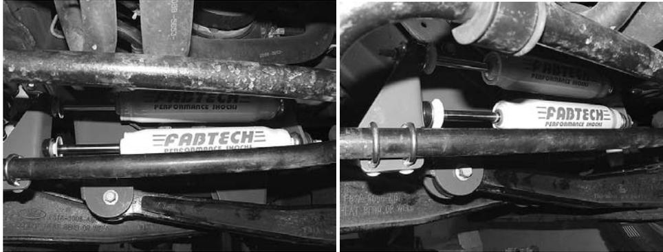
6. Measure both shocks, making sure they are at the center of their stroke. Once everything is positioned properly, Fully tighten the u bolts to 20 ft/lbs.
