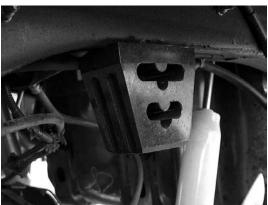
Remove the OEM rear bump stops and replace them with the new urethane units. Use the included 3/8" hardware
