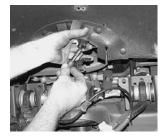
12. Route the ABS sensor wire onto the UCA the same way it was removed. Reattach the wire to the UCA and shock keepers. Reconnect the wire behind the inner fender. You may have to slide the rubber insulators on the sensor wire to relocate them in the clamps. You may have to use some light oil to aid in moving the insulators.
