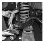
9. Take the passenger's side lift spindle and slide it onto the upper and lower ball joints. Reinstall the original castle nuts. Torque the castle nuts to factory specifications and install 2 of the supplied new cotter pins. Grind lip 1/8" on (LCA) to clear spindle.
