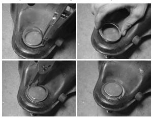
8. Remove the snap ring from the top of the lower ball joint. Place one FT97159-7-101 shim over the ball joint and replace the snap ring on the lower ball joint, making sure the snap ring is fully seated in the groove.
