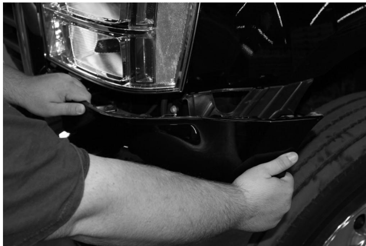
Figure 3 - Plastic Section Removal
