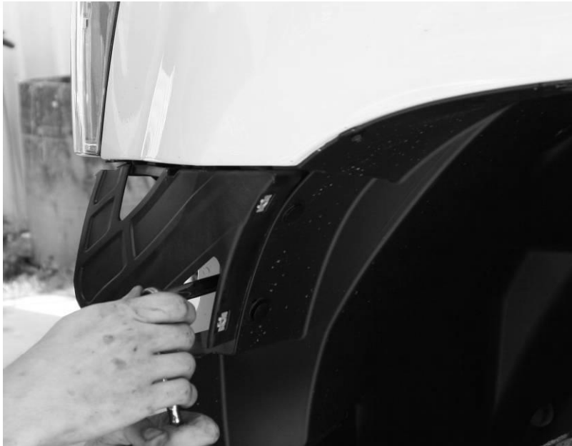
Figure 6 - Support Bracket Removal
