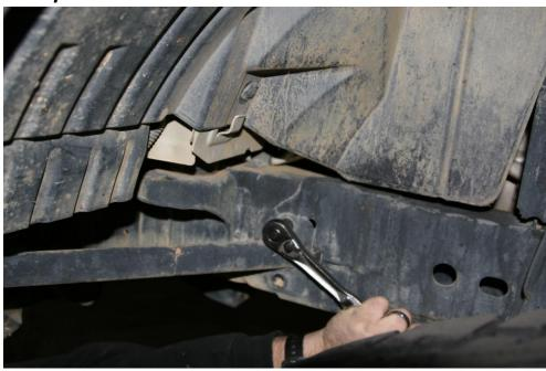
D. Using a 14mm socket and extension remove the bolt located inside the tow hook area on either side.
