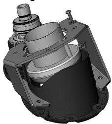
D. Install light pocket into bumper through front face, align corresponding fog lamp/bracket from back side. Secure with 10 (each side) button head screws as shown. Verify that light alignment adjusters are on bottom of light assembly. Repeat for other side.
