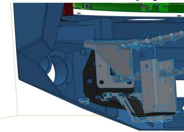
G. Using either the help of friends or a wood block on a floor jack under the bumper, locate the bumper to a .5"gap below the grill and headlights. Also align the bumper to the fenders from the side. Fully Tighten All bolts.
