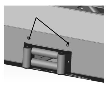
E. Install the Frame mounts to the frame using the supplied 7/16" hardware as shown below using a lock washer and two washers per bolt and nut. Do not Fully Tighten.
