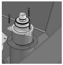
I. Install fog lamp brackets onto inner light pockets using two bolts and nuts per side and attach running light to bracket as shown using two bolts, washers, and nuts per side. Verify that light adjustment screw is facing downward before tightening fully.
