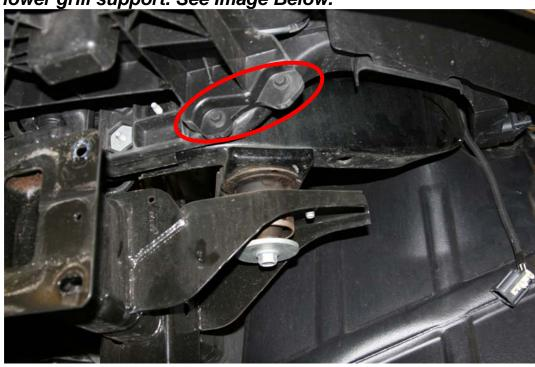
G. Remove the 4 10mm bolts holding the grill into place, and remove the grill
