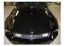
STEP 5: Align stripes on hood by using holes cut for window washers and center marks placed at front of hood. Liner/backing of stripes should line up to each other as shown below.
