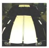
STEP 6: After aligning hood stripes, tape and "hinge" one side of stripe in place and install to hood as shown below. Repeat for other side using liner/backing and window washer holes for alignment. Ends of stripes at front and rear of hood should be rolled under edges and securely adhered.
