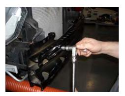
STEP 14: Install (4) nuts on rear side of bumper bolts and tighten down onto the splitter bracket to 18 ft.-lb.
