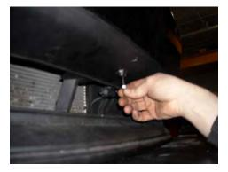
**STEP 36:** Install the splitter support rods onto rod ends; torque bolts through splitter to 28 in.-lb.
