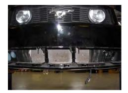
**STEP 23:** Slide the lower grill insert into fascia and clip into place.
