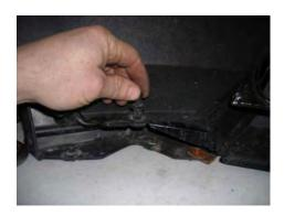
**STEP 17:** Gently unclip lower grill insert from fascia and remove by sliding forward.
