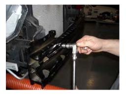
STEP 12: Install the new splitter bracket over bumper and slide onto lower (2) bumper bolts.
