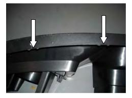
STEP 27: Slide the provided J-Nuts onto the (8) locations and transfer the locations for the new holes.
