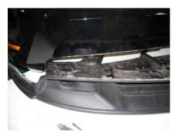
**STEP 18:** Place templates on top side of lower grill insert and transfer hole locations.
