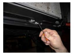
STEP 21: Replace the removed clips with the (4) J-Nuts provided in Splitter Kit M-16601P-MB.
