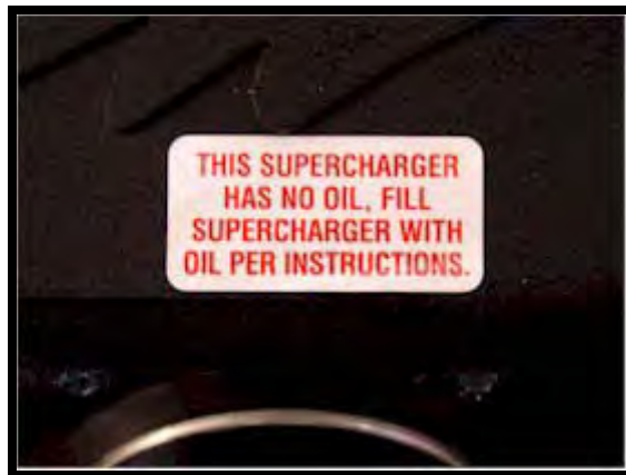
Warning label attached to Supercharger housing
