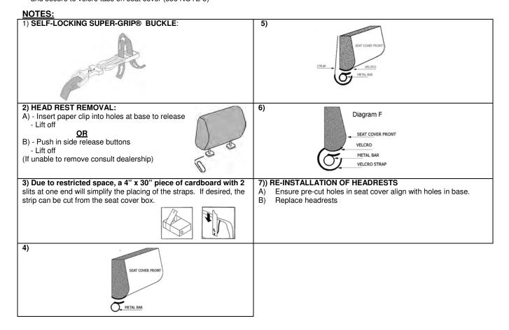
WARNING: NEVER INSTALL SEAT COVERS ON SEATS WITH BUILT-IN AIRBAGS AS THIS MAY INTERFERE WITH THE PROPER DEPLOYMENT OF THE AIR BAGS WHICH COULD RESULT IN SERIOUS INJURY.
