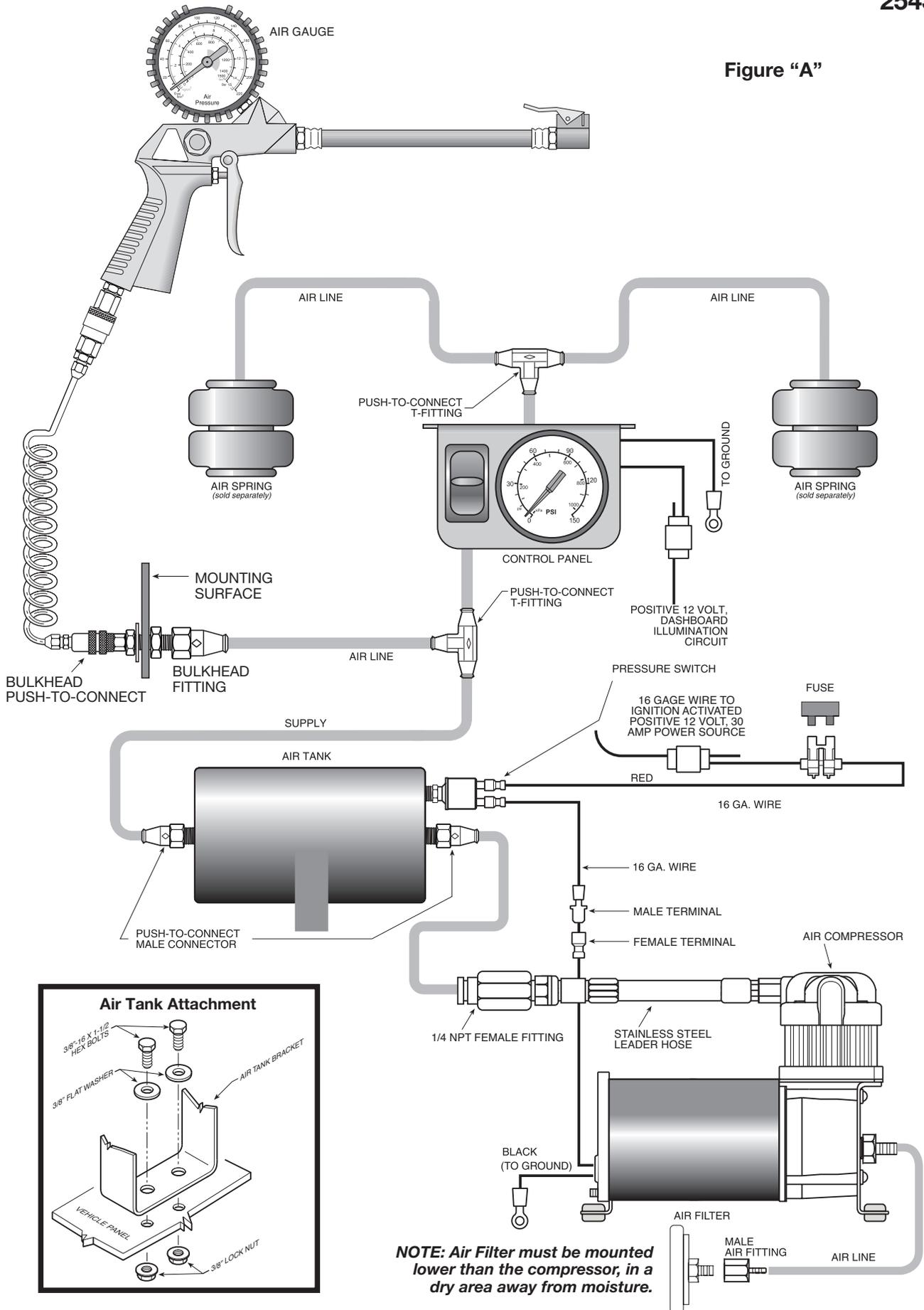
**NOTE: Air Filter must be mounted lower than the compressor, in a dry area away from moisture.**
