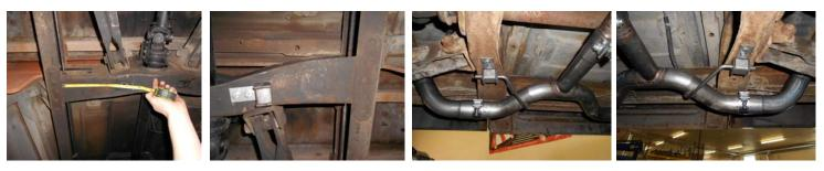
2) Take the right and left H-pipe assemblies, **86074** & **86075** and connect them together at the center cross-over connection. Place them up into position and connect the hangers on the pipe to the rubber mounts installed above. The hanger rods should stick thru the rubber block on the **HA572** hanger approx. 1.00". Support the front of the assembly with a stand. Place the provided 2" clamp at the center H-pipe connection.
