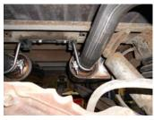
6) Place a supplied clamp onto the right muffler outlet; take the right over-axle tailpipe **#86077** and slide into the muffler outlet while connecting the front hanger on the pipe to the rubber mount installed in step 3 above. The tailpipes have been left long to work for long bed model trucks, for short bed trucks the rear of the tailpipes will need to be trimmed approximately 12.00". Place a second **HA572** hanger onto the rear hangers in preparation for the two steps below.
