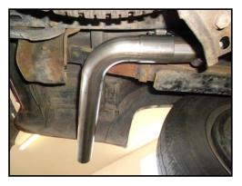
7) Included in the system are 2 different exit pipe styles, determine which of the exit pipes that you would like to use. Place a clamp over the expanded end of your chosen exit pipe and slide them onto the back of the over-axle pipes. Tighten the clamps enough to hold. **Note:** For short bed model trucks, 10.00" will need to be trimmed from the back of the rear exit pipes #86357 & #86358.
