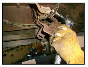
2) Remove the factory pipe hangers from the front and middle exhaust hanger mounts.
