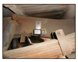
2) Locate the cross member at the front of the rear leaf spring, on the left side of this cross member, there will be a factory hole  $9.00^\circ$  in from the frame and  $34^\circ$  up from the bottom, this hole location will need to be duplicated on the right side of the vehicle. Measure over  $9.00^\circ$  from the frame and  $34^\circ$  up as shown in the photos below, use a center punch to make a mark and drill a  $5/16^\circ$  hole on this mark.
