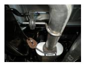
6) Connect the inlet of the muffler **#8530572-Z** to the inlet pipe. Use a stand to support the muffler and install clamp hanger **#392HA** provided in the parts kit onto the inlet of the muffler. Tighten the clamp enough to hold but still allow for adjustment.
