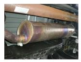
3) Loosen the factory clamp from the inlet of the muffler. Once the clamp is loose, the connection may need to be heated with a torch to ease removal. *Be extremely careful when using a torch.*
