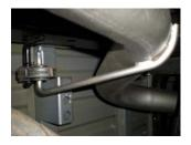
5) Install tailpipe **#26338S** by guiding it into the stock location, up and over the rear of the axle housing and into the back of muffler. Connect the wire hanger on the tailpipe to the factory rubber mount at the rear of the vehicle. Slide stainless tip **#ST429** over the rear of the tailpipe.
