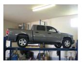
1) Raise the vehicle up on a hoist or rack to working height and support securely with jack stands.
