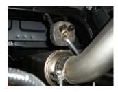
4) Place rear muffler clamp/hanger assembly **#413HA** onto the outlet of the muffler and connect to the rubber mount on the vehicle. Tighten the clamp enough to hold but still allow for adjustment.
