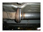
5) Place the flange of inlet pipe **#543TBS** up to the front flange and reinstall the two nuts previously removed. Tighten the nuts evenly to allow the two flange surfaces to be parallel. Tighten enough to hold but still allow for adjustment.
