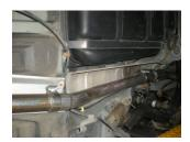
7) Place a provided clamp onto the expanded end of over-axle pipe #16773S and slide onto the back of the mid pipe #16772S. Rotate the pipe up into its approximate position and tighten the clamp enough to hold, but still allow for adjustment.
