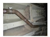
6) Place a provided clamp onto the expanded end of intermediate pipe **#16772S** and slide onto the back of adapter pipe **#555TBS** or inlet pipe **#16771S**. Rotate the pipe up into its approximate position and tighten the clamp enough to hold, but still allow for adjustment.
