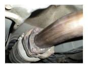
3) If your vehicle is an EX or SI model with the 2.0L engine, remove the three nuts attaching the factory mid pipe to the rear of the catalytic converter. Once the flange is loose, remove the two hangers at the rear of the pipe from the rubber mounts on the vehicle and lower the pipe from the vehicle.
