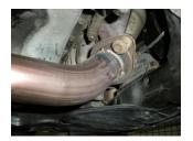
5) For 2.0L models with mid cat, place adapter pipe **#555TBS** onto the back of the catalytic converter and replace the three nuts removed in step 3 above. Tighten securely. For 1.7L models, place inlet pipe **#16771S** onto the bottom of the exhaust manifold and replace the bolts and springs removed in step 4 above. Connect the hanger on the pipe to the rubber mount on the vehicle.
