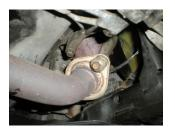
4) If your vehicle is a DX or LX model with the 1.7L engine, remove the two bolts at the flanged connection below the exhaust manifold. Once the flange is loose, remove the two hangers at the rear of the pipe from the rubber mounts on the vehicle and lower the pipe from the vehicle.
