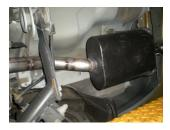
8) Place a provided clamp onto the inlet of muffler #852460-269 and slide the inlet onto the back of over-axle pipe #16773S. Support the muffler with a stand and connect the four hangers on the muffler assembly to the rubber mounts on the vehicle. Tighten the clamp on the muffler inlet enough to hold, but still allow for adjustment.
