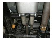
9) Place the front section of the left side tailpipe **#16508S** into the left side muffler outlet and connect the hanger on the pipe to the rubber mount on the vehicle. Tighten the 2 1/2" clamp on the muffler outlet just enough to hold in position.
