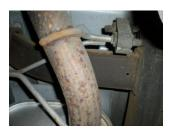
2) Support the muffler with a stand. Using a hacksaw or sawsall, cut the stock tailpipe in front of the rear end behind the muffler hangers. Separate the wire hanger on the tailpipe from the rubber mount on the vehicle and remove the tailpipe from the vehicle.
