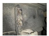
8) To simplify the installation of the rear section of the tailpipe, **#16721S**, remove the rear hanger mount from the frame and slide the hanger assembly onto the hanger of pipe **#16721S**.
