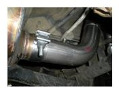
7) Place a provided 2½" clamp onto the muffler outlet and then place the tailpipes front section pipe **#16720S** into position over the axle. Tighten the clamp enough to hold but still allow adjustment.
