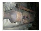
4) Support the muffler with a stand, and with a 15mm wrench remove the muffler clamp at the catalytic converter to muffler connection. Remove the muffler assembly from under the vehicle.
