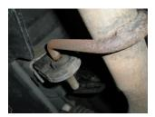
3) Separate the wire hanger on the tailpipe from its rubber mount on the vehicle. Remove the tailpipe and set aside.
