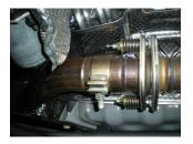
3) Support the front and the rear of the system with a stand. Make your way forward from the rear and remove all of the wire hangers on the system from the rubber mounts on the vehicle. Then at the front flange connections, remove the nuts on the spring bolts and set the hardware aside, the springs and nuts will be reused with the Flowmaster system. With the help of an assistant, you can now lower the stands and remove the entire system from the vehicle and set aside.
