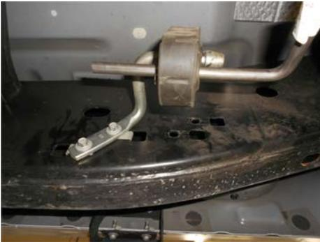
3) Slide clamp hanger **#382HA** over the back of the inlet pipe and insert the hanger into the factory rubber mount bolted to the side of the frame. Do not tighten this clamp yet. If the extension pipe is used, use the provided 3" band clamp at the connection between the inlet and extension pipe. **Note:** If the **382HA** hanger doesn't line up with the rubber mount, the mount may need to be re-located slightly forward and down to the other set of factory mounting holes in the frame.
