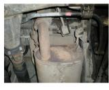
2) Unbolt the tailpipe connection behind the muffler using a 14mm socket or wrench, then remove the factory tailpipe hanger from the rubber mount on the vehicle and set tailpipe aside.
