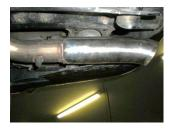
8) Place tailpipe assembly **#16755S** up over the rear axle and into the muffler outlet. Connect the hanger at the rear of the pipe to the rubber mount on the vehicle. Adjust the tip to the desired rotation and tighten the clamp enough to hold but still allow for adjustment. **Note:** Depending on the model year and or spare tire size, the spare tire may need to be dropped down to allow installation of the new Flowmaster tailpipe.
