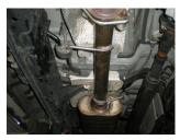
6) Place the supplied  $2\frac{1}{2}$ " clamp onto the inlet of muffler **#852572-Z** and slide onto the inlet pipe and support with a stand. Level the muffler and tighten the clamp enough to hold but still allow for adjustment.
