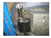
8) Place the **ST339** stainless tip onto the muffler outlet and adjust to the desired position. Tighten the clamp enough to hold, but still allow for adjustment.
