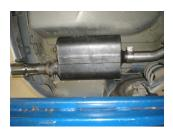
7) Place a provided clamp onto the inlet of muffler #852562-267 and slide the inlet onto the back of over-axle pipe #16769S. Support the muffler with a stand and connect the two hangers on the muffler assembly to the rubber mounts on the vehicle. Tighten the clamp on the muffler inlet enough to hold, but still allow for adjustment.
