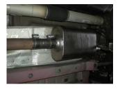
5) Place a provided 2.50" clamp onto the inlet of muffler #852557-Z and slide the inlet onto the back of the adapter pipe #TB556S. Support the muffler with a stand and tighten the clamp on the muffler inlet enough to hold, but still allow for adjustment. The outlet of the muffler will be positioned toward the outside of the vehicle.
