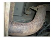
2) Support the muffler with a stand. Using a hacksaw or sawsall, cut the stock tailpipe off just behind the muffler. Separate the wire hangers on the tailpipe from the rubber mounts on the vehicle and remove the tailpipe from the vehicle.
